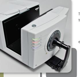
The UltraScan® VIS color measurement spectrophotometer measures opaque, transparent, and translucent solids and liquids in
