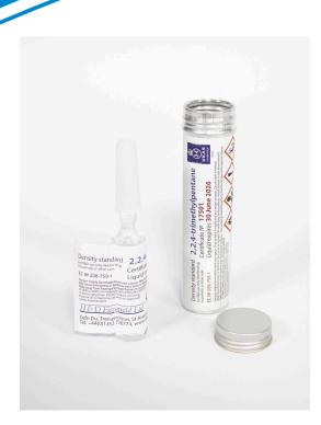
Bellingham + Stanley now supplies certified reference fluid for verifying the performance of digital density meters including the DSG Series Density Meters DSG40 and DSG50.
